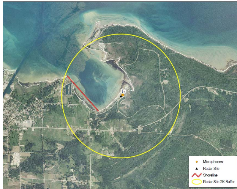
Fig. 4. Example configuration for Site 1S. The radar detects individual flights, with height, to a radius of 2 km (yellow circle). Bat and bird microphones are set in an array (orange circles) to monitor species-specific activity within a subset of the radar volume of detection (100 m from each bat microphone and 600 m from each bird microphone). A line is drawn along the shore within the radar volume of detection for analysis of activity and behaviour along the shore versus an equal length line, drawn at the same orientation, within the paired inland plot.
