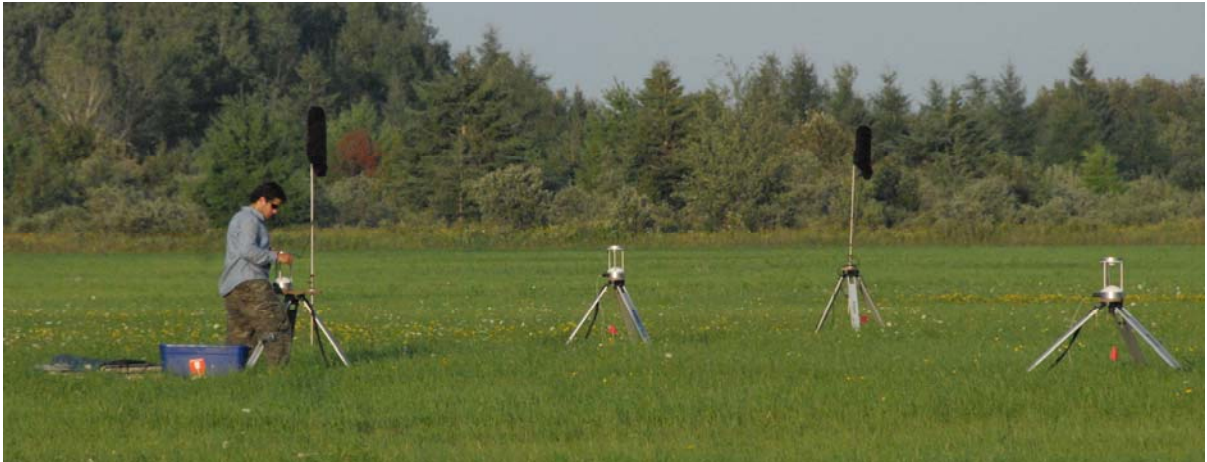
Fig. 3. Within plot sampling protocol. The radar is trailer mounted and the bird and bat microphones are set on tripods in an array that is 75 m in a field perpendicular to the trailer.
